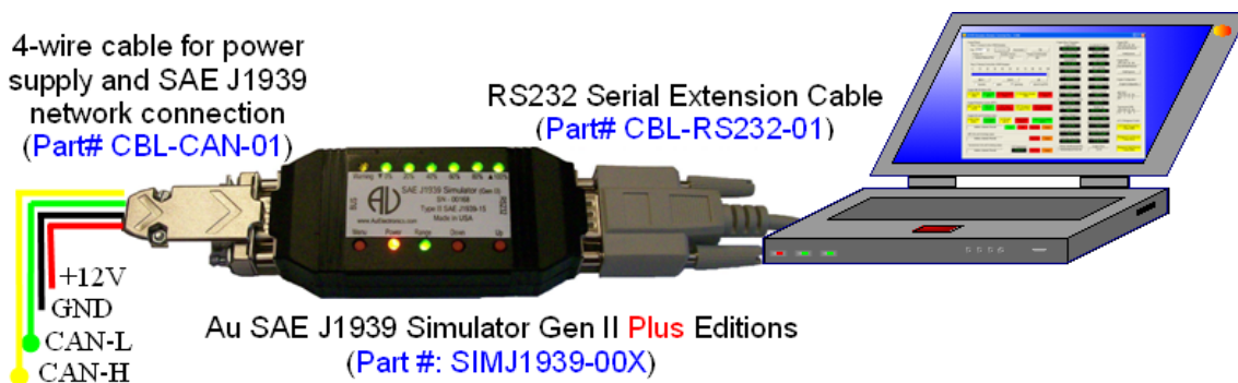
Figure 1-5 Connection of Au J1939 Simulator (Gen II) plus editions to PC with RS232 port
