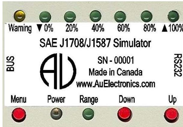
Figure 2-1 Push buttons and LEDs on Au J1708 Simulator
