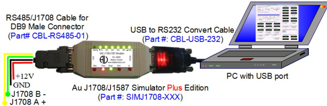
Figure 1-6 Connection of J1708/J1587 Simulator plus editions to PC with USB port
