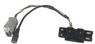
The DB9 female connector can be connected with Au Group Electronics OBD2 CAN simulators. It will supply power, ground, CAN-H, CAN-L, to Au Group Electronics developed OBD2 CAN devices.
