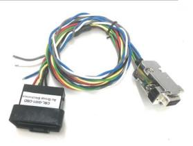
Power, Ground, CAN\_H, CAN\_L are connected from / to the vehicle via this OBD-II male housing.
